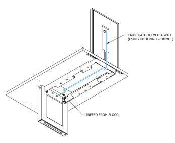
CABLING DIAGRAM: WALL-MOUNTED TABLE AND PARTIAL MEDIA WALL WITH TABLETOP POWER OPTION
